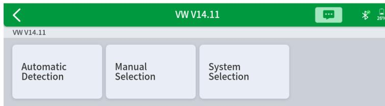
Automatic Detection will automatically identify the vehicle's VIN code, and then read the information of your target diagnostic object. If you choose "Manual selection", then you can continue to select the vehicle brand, year, and model of the vehicle in the sub-menu to diagnostic the vehicle. Enter "System Selection", you can also diagnose the vehicle according to the system according to your needs after selecting the model.
